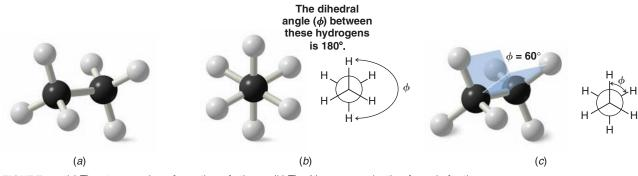
**FIGURE 4.5** (*a*) The staggered conformation of ethane. (*b*) The Newman projection formula for the staggered conformation. (*c*) The dihedral angle between these hydrogen atoms is 60°.
