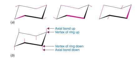
**FIGURE 4.18** (*a*) Sets of parallel lines that constitute the ring and equatorial C - H bonds of the chair conformation. (*b*) The axial bonds are all vertical. When the vertex of the ring points up, the axial bond is up and vice versa.
