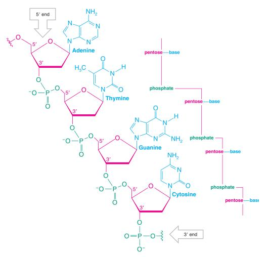
**FIGURE 25.7** A segment of one DNA chain showing how phosphate ester groups link the 3'- and 5'-OH groups of deoxyribose units. RNA has a similar structure with two exceptions: a hydroxyl replaces a hydrogen atom at the 2' position of each ribose unit and uracil replaces thymine.
