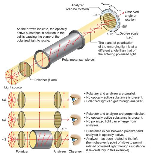
FIGURE 5.12 The principal working parts of a polarimeter and the measurement of optical rotation. (Reprinted with permission of John Wiley & Sons, Inc. from Holum, J. R., *Organic Chemistry: A Brief Course*, p. 316. Copyright 1975.)
