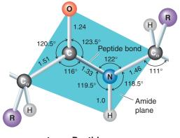
**FIGURE 24.9** The geometry and bond lengths (in angstroms, Å) of the peptide linkage. The six enclosed atoms tend to be coplanar and assume a "transoid" arrangement. (Reprinted with permission of John Wiley & Sons, Inc., from Voet, D. and Voet, J. G., *Biochemistry*, Second Edition. © 1995 Voet, D. and Voet, J. G.)
