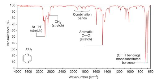
FIGURE 2.12 The IR spectrum of methylbenzene (toluene).
