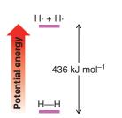
**FIGURE 3.7** The relative potential energies of hydrogen atoms and a hydrogen molecule.
