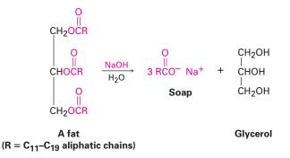
Crude soap curds contain glycerol and excess alkali as well as soap but can be purified by boiling with water and adding NaCl or KCl to precipitate the pure carboxylate salts. The smooth soap that precipitates is dried, perfumed, and pressed into bars for household use. Dyes are added to make colored soaps, antiseptics are added for medicated soaps, pumice is added for scouring soaps, and air is blown in for soaps that float.
