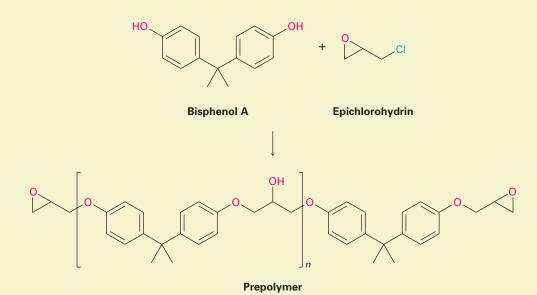
When the epoxide is to be used, a basic curing agent such as a tertiary amine,  $R_3N$ , is added to cause the individual prepolymer chains to link together. This "cross-linking" of chains is simply a base-catalyzed,  $S_N2$  epoxide ring-opening of an -OH group in the middle of one chain with
