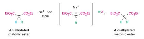
On heating with aqueous hydrochloric acid, the alkylated (or dialkylated) malonic ester undergoes hydrolysis of its two ester groups followed by *decarboxylation* (loss of  $CO_2$ ) to yield a substituted monocarboxylic acid. Decarboxylation is a unique feature of compounds like malonic acids that have a second carbonyl group two atoms away from the  $-CO_2H$  and is not a general reaction of carboxylic acids.
