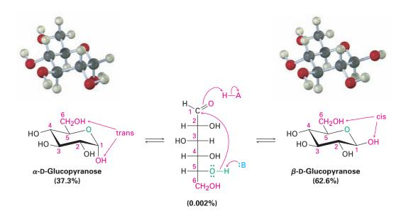
The minor anomer, which has the C1 –OH group trans to the –CH<sub>2</sub>OH substituent at C5, is called the **alpha** ( $\alpha$ ) **anomer**; its full name is  $\alpha$ -D-glucopyranose.
