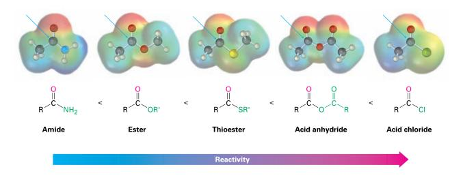
A consequence of these reactivity differences is that it's usually possible to convert a more reactive acid derivative into a less reactive one. Acid chlorides, for example, can be converted into esters and amides, but amides and esters can't be converted into acid chlorides. Remembering the reactivity order is therefore a useful way to keep track of a large number of reactions (Figure 10.3).
