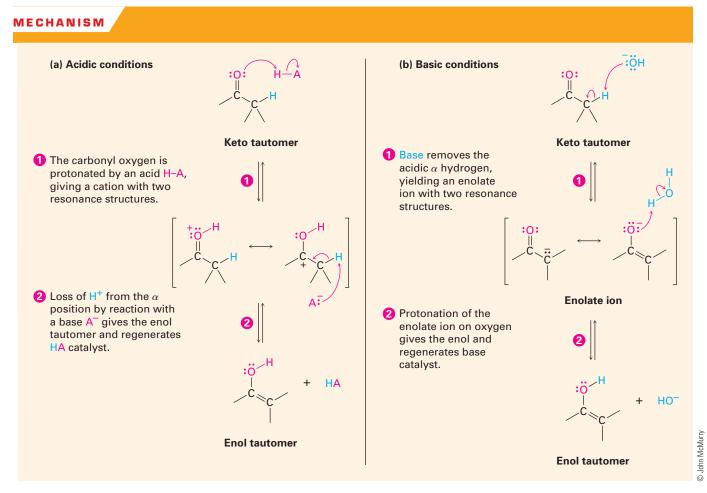
**Figure 11.1** Mechanism of enol formation under both acid-catalyzed and base-catalyzed conditions. (a) Acid catalysis involves initial protonation of the carbonyl oxygen followed by removal of H<sup>+</sup> from the  $\alpha$  position. (b) Base catalysis involves initial deprotonation of the  $\alpha$  position to give an enolate ion, followed by reprotonation on oxygen.
