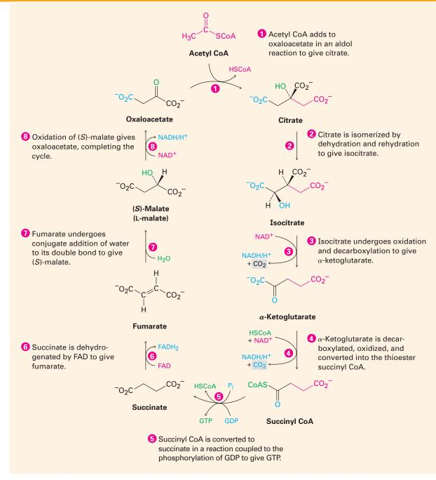
**Figure 17.5** The citric acid cycle is an eight-step series of reactions that results in the conversion of an acetyl group into two molecules of CO<sub>2</sub> plus reduced coenzymes. Individual steps are explained in the text.
