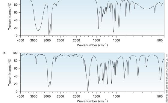
One further point about infrared spectroscopy: it's also possible to obtain structural information from an IR spectrum by noticing which absorptions are *not* present. If the spectrum of an unknown does *not* have an absorption near 3400 cm<sup>-1</sup>, the unknown is not an alcohol; if the spectrum does not have an absorption near 1715 cm<sup>-1</sup>, the unknown is not a ketone; and so on.
