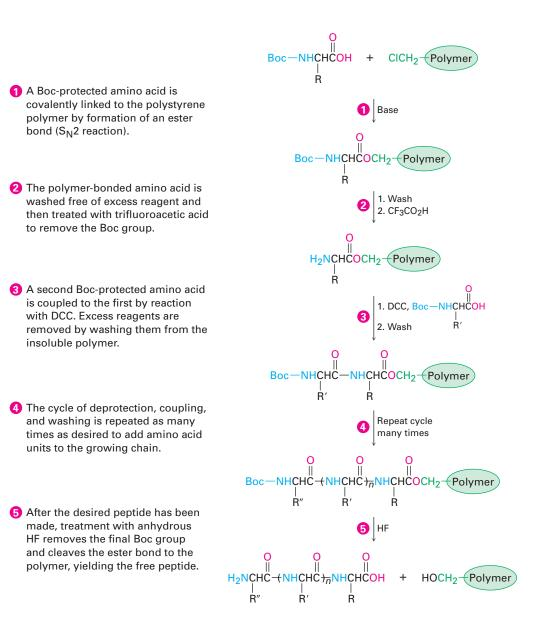
Robotic peptide synthesizers automatically repeat the coupling, washing, and deprotection steps with different amino acids. Each step occurs in high yield, and mechanical losses are minimized because the peptide intermediates are never removed from the insoluble polymer until the final step. Using this procedure, up to 30 mg of a peptide with 20 amino acids can be routinely prepared in a few hours.
