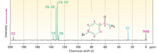
**Figure 13.16** The  ${}^{13}$ C NMR spectrum of *p*-bromoaceto-phenone, BrC<sub>6</sub>H<sub>4</sub>COCH<sub>3</sub>.
