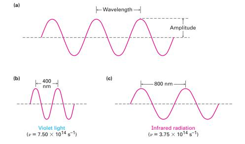
Multiplying the length of a wave in meters (m) by its frequency in reciprocal seconds (s<sup>-1</sup>) gives the speed of the wave in meters per second (m/s). The rate of travel of all electromagnetic radiation in a vacuum is a constant value, commonly called the "speed of light" and abbreviated *c*. Its numerical value is defined as exactly 2.997 924 58 × 10<sup>8</sup> m/s, usually rounded off to  $3.00 \times 10^8$  m/s.
