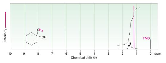
spectrum of the reaction product from H<sub>2</sub>O and 1-methylcyclohexene. The presence of the  $-CH_3$ absorption at 1.19  $\delta$  and the absence of any absorptions near 4  $\delta$  identify the product as 1-methylcyclohexanol.
