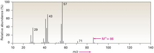
In addition to giving a molecular ion, most molecules fragment in the mass spectrometer, giving rise to numerous other ions that can provide structural information when interpreted. Hexane, for instance, shows peaks at m/z = 71 corresponding to loss of a CH<sub>3</sub>– group, m/z = 57 corresponding to loss of an CH<sub>3</sub>CH<sub>2</sub>– group, m/z = 43 corresponding to loss of a CH<sub>3</sub>CH<sub>2</sub>– group, and so forth.
