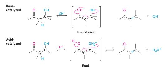
The reaction conditions needed for aldol dehydration are often only a bit more vigorous (slightly higher temperature, for instance) than the conditions
