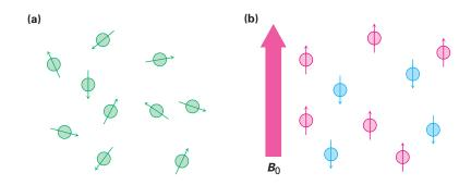
**Figure 13.8** (a) Nuclear spins are oriented randomly in the absence of an external magnetic field but (b) have a specific orientation in the presence of an external field  $B_0$ . Some of the spins (red) are aligned parallel to the external field and others (blue) are antiparallel. The parallel spin state is lower in energy and therefore favored.
