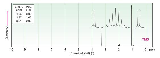
**13.73** Propose structures for compounds that fit the following <sup>1</sup>H NMR data: (a)  $C_4H_6Cl_2$  (b)  $C_{10}H_{14}$
