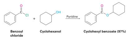
Because HCl is generated as a by-product, the reaction is usually carried out in the presence of an amine base such as pyridine (see Section 12.6), which reacts with the HCl as it's formed and prevents it from causing side reactions.
