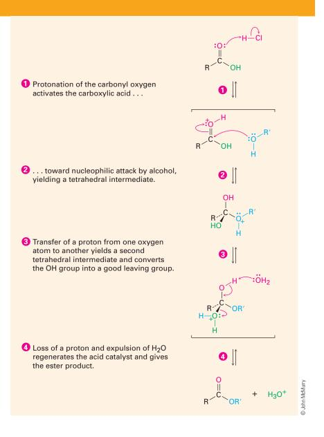
All steps in the Fischer esterification reaction are reversible, and the position of the equilibrium can be driven either forward or backward depending on the reaction conditions. Ester formation is favored when alcohol is used as the solvent, but carboxylic acid is favored when the solvent is water.
