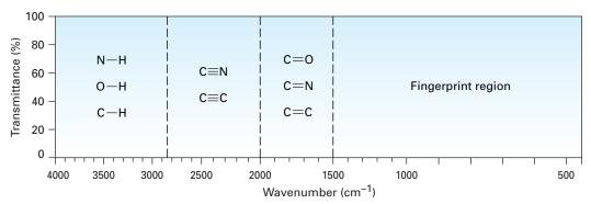
• The region from 4000 to 2500 cm<sup>-1</sup> corresponds to absorptions caused by N–H, C–H, and O–H single-bond stretching motions. N–H and O–H bonds absorb in the 3300 to 3600 cm<sup>-1</sup> range; C–H bond stretching occurs near 3000 cm<sup>-1</sup>.
