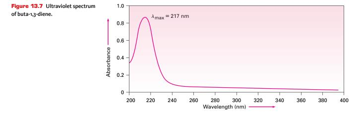
The amount of UV light absorbed by a sample is expressed as the sample's absorbance (A), defined by the equation
