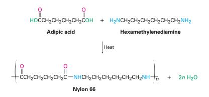
Nylons are used both in engineering applications and in making fibers. A combination of high impact strength and abrasion resistance makes nylon an excellent metal substitute for bearings and gears. As fiber, nylon is used in a variety of applications, from clothing to tire cord to ropes.
