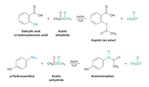
Notice in both of these examples that only "half" of the anhydride molecule is used; the other half acts as the leaving group during the nucleophilic acyl substitution step and produces carboxylate anion as a by-product. Thus, anhydrides are inefficient to use, and acid chlorides are normally used instead.
